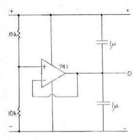
The non-inverting input of the 741 is at half the supply potential, so for example if the input is at 20 V, the three output terminals will be  $\pm 10$  V, 0 V and  $\pm 10$  V.
