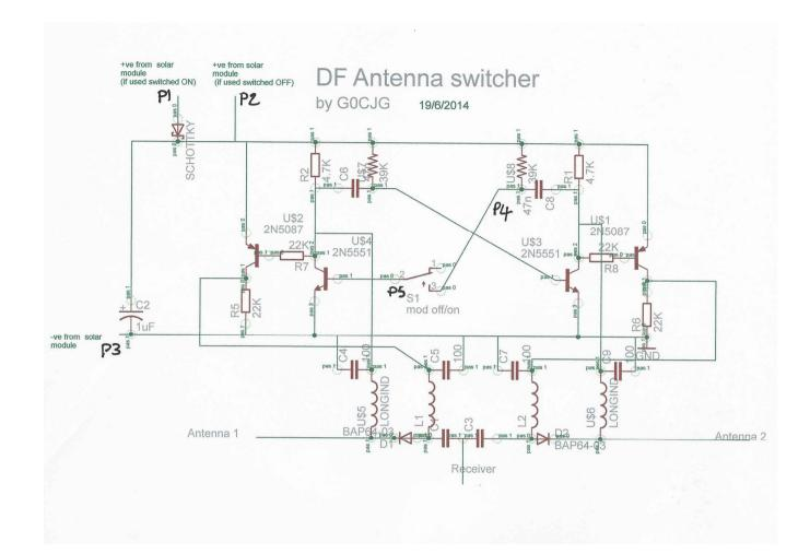
P1 +ve from solar (Solar ON) P2 +ve from solar (Solar OFF) P3 –ve from Solar P4,P5 Modulation on/off switch Wire P4,P5 together if switch not used
